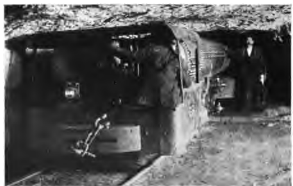
Fig. 6. Pneumatic Engine used to Avoid Danger of Fire.*
